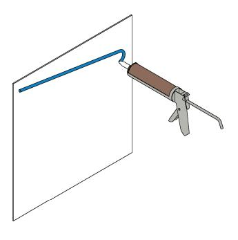
4) Working quickly, complete the Wall Tile in a back-and-forth pattern as shown below.
